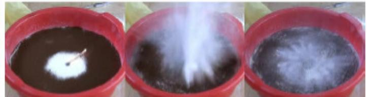
Fig. 1: Our explosion-induced laboratory craters were produced in stone powder using silver acetylide ( $\text{Ag}_2\text{C}_2$ ) as the explosive. The powder was compressed such that the surface density was 1.60–1.75 g/cm<sup>3</sup>. The charge mass varied from 10mg to 635mg. The explosive was positioned just below the surface.
