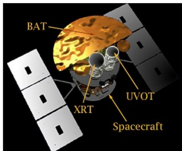
Figure 2.1: The *Swift* spacecraft with its three telescopes: Burst Alert Telescope (15 – 150 keV, FOV 2 sr), X-ray Telescope (0.3 – 10 keV, FOV  $23.6'' \times 23.6''$ ) and UV/Optical Telescope (180 – 600 nm, FOV  $17'' \times 17''$ ). Taken from <https://www.swift.psu.edu>.
